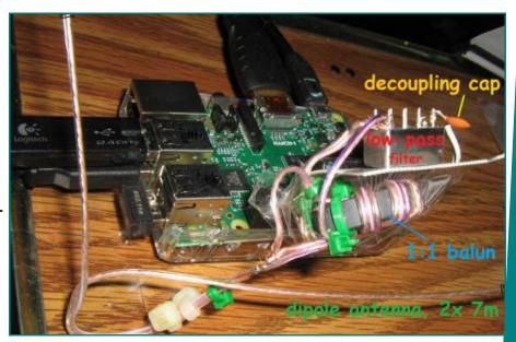
The software he chose is WsprryPi (https://github.com/JamesP6000/WsprryPi). It's described a "Raspberry Pi transmitter using NTP-based frequency calibration." It uses a GPIO port to generate WSPR signals anywhere from 0 to 250 MHz. Joe said that there are several Raspberry Pi programs that run WSPR, but that he chose this one because it seemed to have more features than the others.
