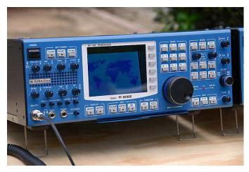
ICOM <<u>http://www.icomamerica.com/</u>> unveiled its IC-7700 HF + 6 meter transceiver. It appears to be a single-receiver version of its top-tier IC-7800, sharing the 200 W transmitter, high performance receiver and 7-inch display of its sibling. Contesters are the market target, but the IC-7700 may be of interest to anyone who covets the features of the IC-7800 but doesn't need two receivers or the higher price tag.
