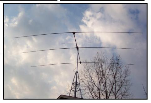
covers ALL frequencies between 20m and 6m inclusive so now I have an three element beam for the WARC bands and four elements (one passive) on 6m.
