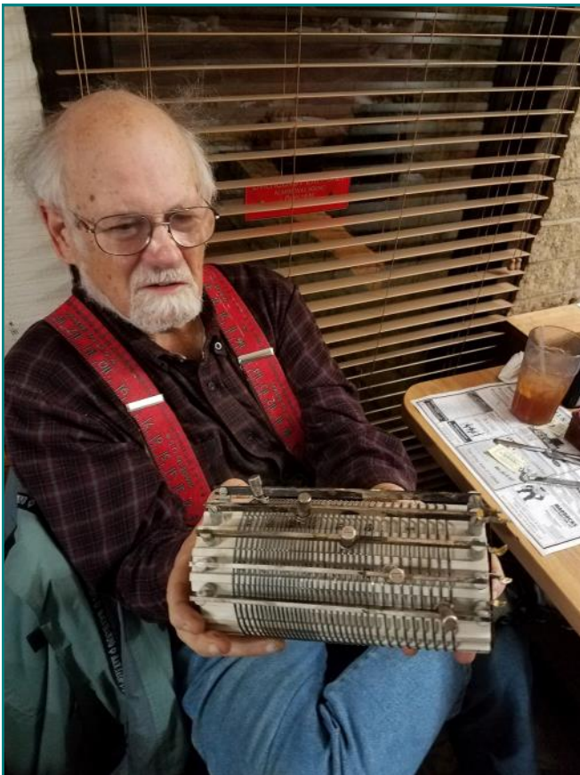
Pete, N8TR, showed off his old large silver plated General Electric fixed inductor that has variable taps for tuning. He purchased this for $2.00 at the 2014 Cleveland Hamfest.
